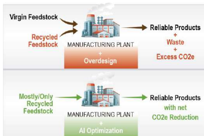
Figure 5-2. AI enables manufacturers to adapt to recycled feedstock. Factories typically address the increased variability of recycled feedstock by planning for the “worst case” scenario; this leads to unnecessary waste and excess emissions. Instead, factories can use AI to optimize operations and produce equally reliable products with net CO 2 e reductions.
