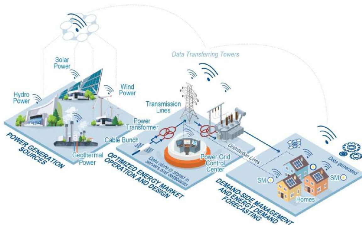
Figure 3-2. Power grid with data transfer
